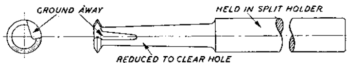
Fig. 5. Form of tool recommended for small internal screwcutting.
