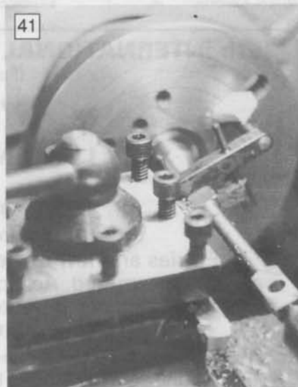
41: Roughing down the connecting rod shank. Note the wooden wedge to prevent the carrier rattling in the slot.
