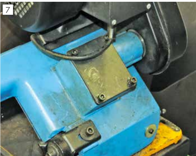
If you are brave, remove this cover, but be prepared for oil spill!
