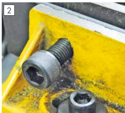
A large bolt used to help balance jaw forces on short workpieces.
