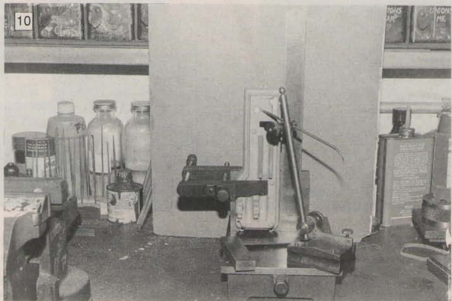
10: Marking out for the cylinder retaining bolt-holes, the casting clamped to an angle plate. 11: Initial alignment of the casting, before drilling for main bearings.
