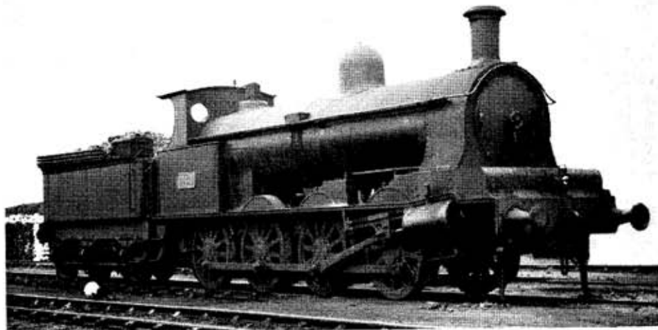
Webb's 4-cylinder compound 0-8-0, of which 170 were built between 1901 and 1904.
