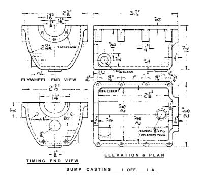
side faces of the housings and caps can be trued up, using a suitable cutter in the boring bar. It will be necessary to replace the sump, and mount the assembly on a stub mandrel, to machine the recesses at both ends and finish the end faces.
