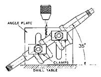
Drilling oil passages in crankshaft
