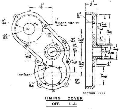
in the body are specified as 1/8 in. Whit., but as studs or bolts of this size are not easy to obtain nowadays, 4 BA, which is some 15 thou larger, may be substituted.
